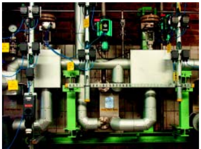
SIGMAWIG ST12 in a heating-cooling circuit for tempering of chemical reactor
